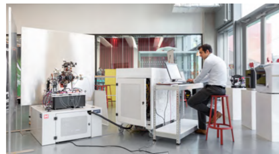
M Squared developed the UK's first commercial quantum accelerometer for navigation applications.
